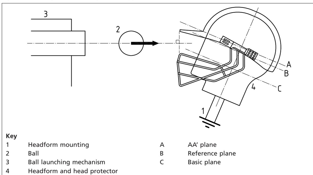
**D.2.1** A headform mounting, permitting independent rotation of the headform in the vertical longitudinal plane and about the central vertical axis by the angle specified in Figure D.4.
