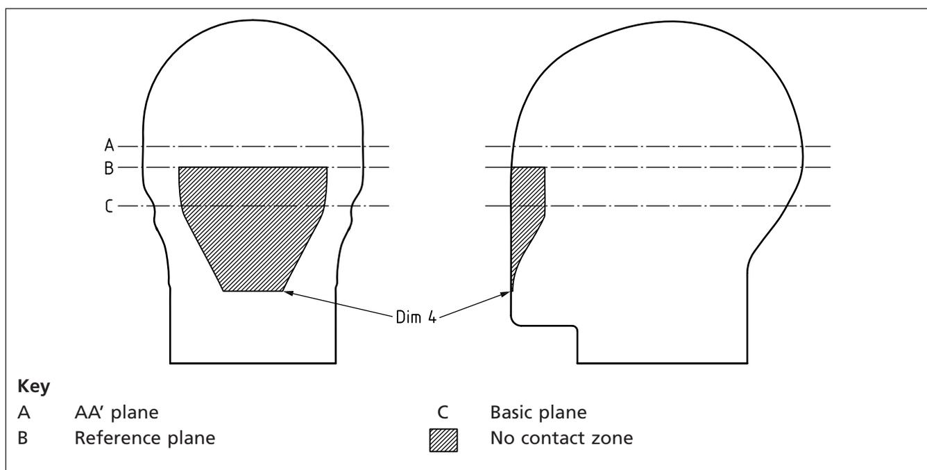
Table D.1 Dimensions of the facial no contact zone for different sized head forms
